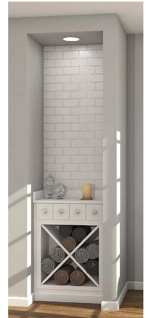
TOWEL CUBBIE CABINET -FULL REAR WALL OF TILE TO MATCH SHOWER SELECTION -WOOD TOP WITH BACKSPASH -RECESSED LIGHT INCLUDED
