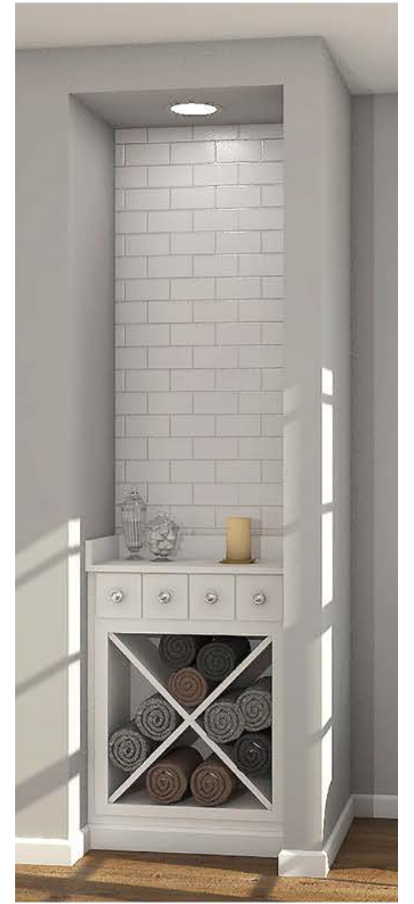
TOWEL CUBBIE CABINET -FULL REAR WALL OF TILE TO MATCH SHOWER SELECTION -WOOD TOP WITH BACKSPASH -RECESSED LIGHT INCLUDED
